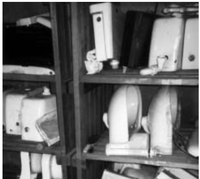
15a Asbestos-reinforced plastic toilet cistern.
