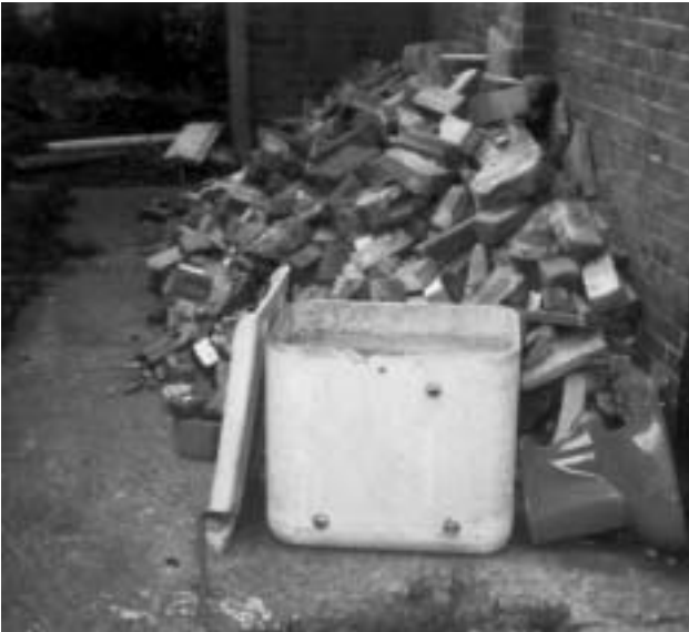
11a Asbestos cement water tank.
