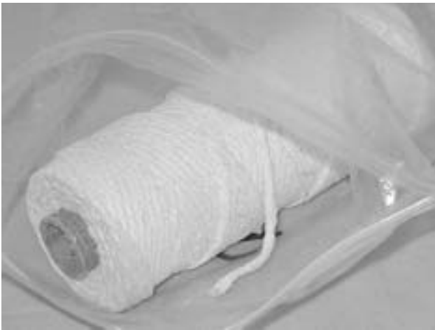
9b Asbestos string.
