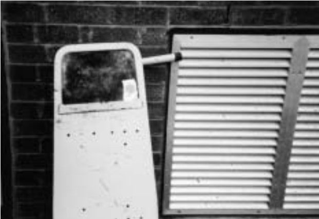
18a Ironing board with asbestos cement sheet for iron rest.
