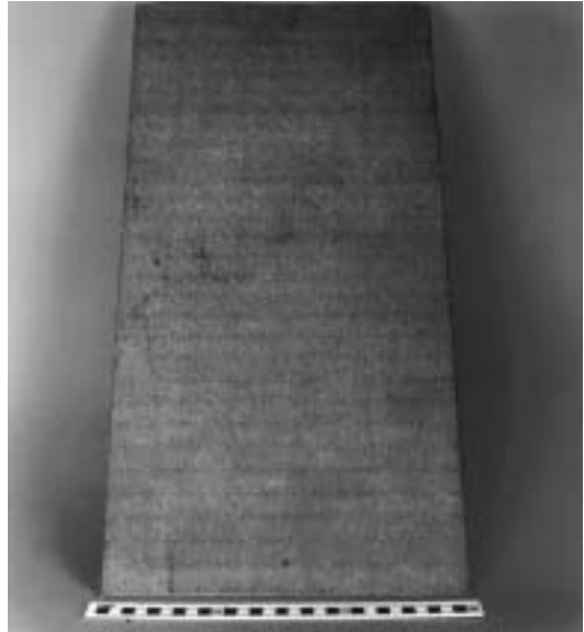
10d Asbestos cement roofing slate.
